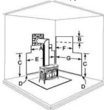
A = 36" (914 mm) B = 13" (330 mm) C = 35" (889 mm) D = 1" (25 mm) E = 40" (1016 mm) F = 30" (762 mm) G = 44" (1118 mm)
